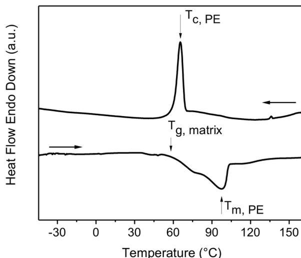
**Figure 3.** DSC thermogram in heating and cooling scans at 10 °C/min for the cured blend with 10 wt % PE-*b*-PEO. [Puig, J.; Zucchi, I. A.; Ceolín, M.; Schroeder, W. F.; Williams, R. J. J. *RSC Adv* **2016**, 6 (41), 34903-34912] Reproduced by permission of The Royal Society of Chemistry.
