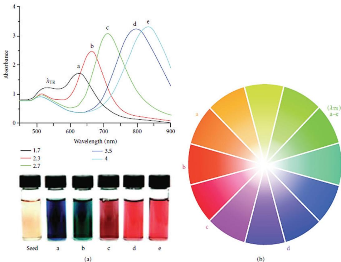
**Figure 5.** Tunable optical properties of gold nanorods (AuNRs) with absorptions at visible and near-infrared wavelengths region. **(a)** Optical absorption spectra of AuNRs with different aspect ratios and composition (a–e). **(b)** Color wheel representing AuNRs labeled a–e, TR = transverse resonance. Reproduced with permission from reference (Tong *et al.* 2009) with permission from John Wiley and Sons and Copyright Clearance Center.
