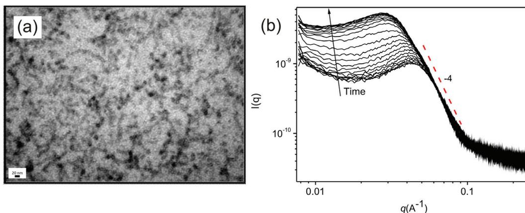
**Figure 13.** (a) TEM image of the epoxy blend with 10 wt % PEB-*b*-PEO fully cured at 80°C. The specimen was stained with RuO<sub>4</sub> prior to TEM observation. Scale bar 20 nm. (b) *In situ* SAXS data obtained during curing at 80°C of the epoxy blend with 10 wt % PEB-*b*-PEO. [Puig, J.; Ceolín, M.; Williams, R. J. J.; Schroeder, W. F.; Zucchi, I. A. *Soft Matter* **2017**, *13* (40), 7341–7351] Reproduced by permission of The Royal Society of Chemistry.
