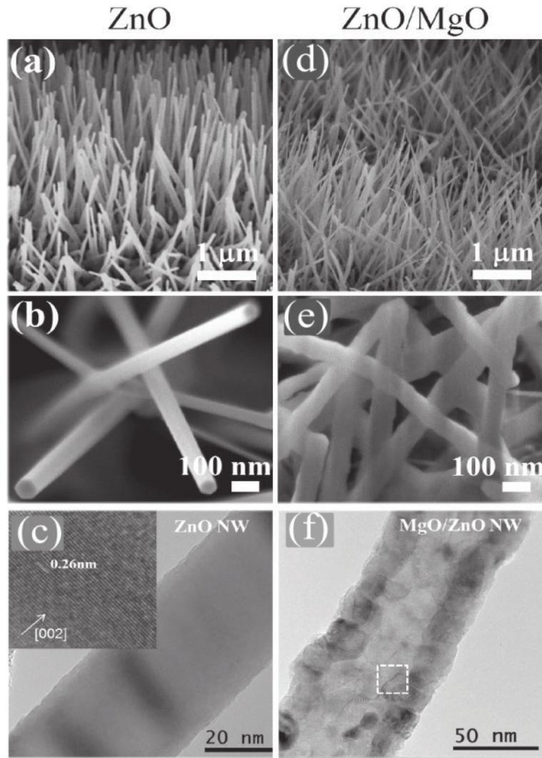
**Figure 6.** SEM images with different magnifications of a ZnO NW sample (a), (b) and of a ZnO/MgO core/shell NW sample (d), (e). As observed in (b), the ZnO NWs are highly crystalline, exhibiting hexagonal cross-section expected from wurtzite c-axis alignment. (c) and (f) show HRTEM images of a ZnO NW and of a ZnO/MgO core/shell NW, respectively. From<sup>76</sup>.
