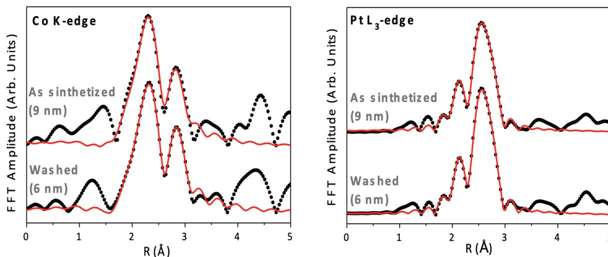
**Figure 1.** Experimental and fitted EXAFS Fourier Transform of fresh and washed NP samples at Co K and Pt L<sub>3</sub>-edges (left and right panels, respectively). Red lines correspond to the EXAFS fitting (see Table 2 for fitted parameters).
