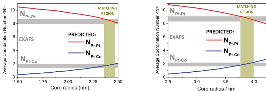
**Figure 3.** Calculated average coordination numbers,  $N_{Pt-Pt}$  (red line) and  $N_{Pt-Co}$  (blue line) as a function of CoPt<sub>3</sub> core radius NP as prepared and washed (left and right panel respectively). The grey horizontal bars represent the average coordination numbers derived from the EXAFS fits. The vertical bar indicates range of the CoPt<sub>3</sub> core radius NP that allows obtaining the coordination numbers matching the experimental data.
