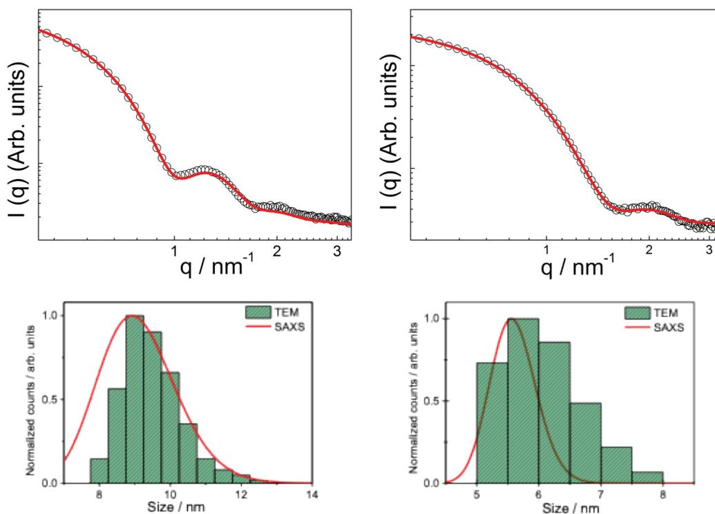
**Figure 5.** Experimental SAXS data (intensity vs. wave vector  $q$  - open symbols) for as-prepared and washed NPs (upper left and right panels, respectively) and the fitting curve obtained based on a spherical core/shell model. The size distributions reconstructed from fitting curve were overlapped with size distribution data obtained based on TEM data (lower panels).
