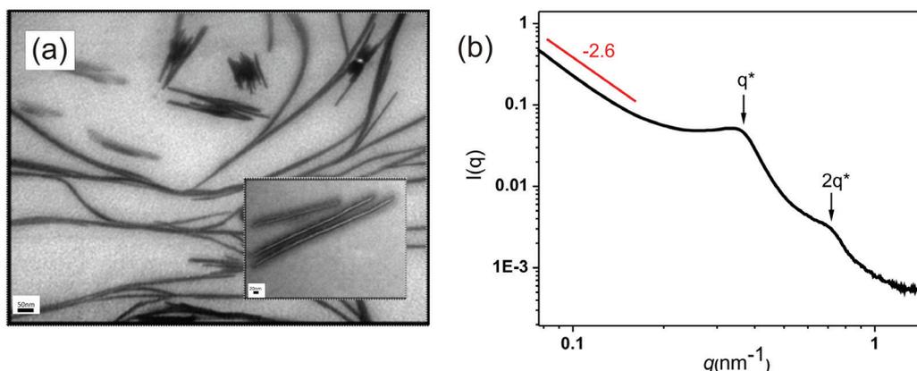
**Figure 4. (a)** TEM images of  $\text{RuO}_4$ -stained section of the photocured blend with 10 wt % PE-*b*-PEO, scale bar 50 nm. **Inset:** TEM image of the same sample at a higher magnification, scale bar 20 nm. **(b)** SAXS profile of the photocured blend with 10 wt % PE-*b*-PEO.
