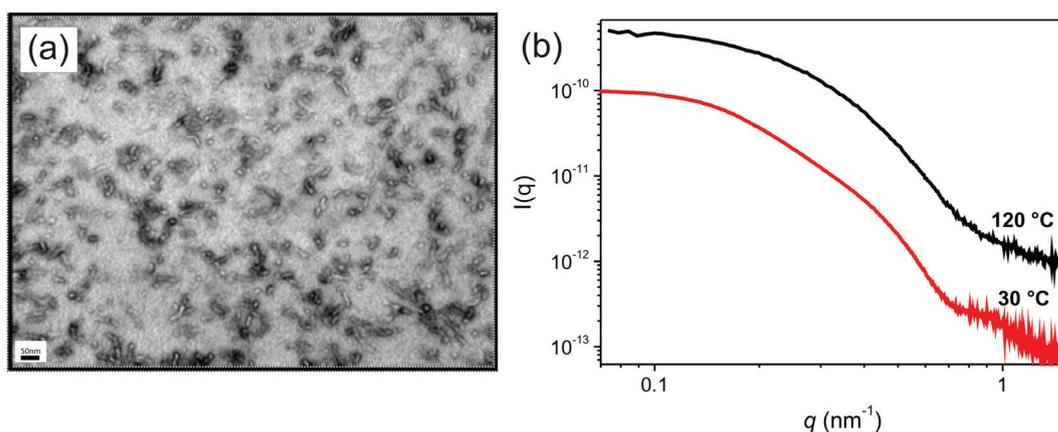
**Figure 2.** (a) TEM image of the fully cured blend containing 10 wt % PE-*b*-PEO, scale bar 50 nm. (b) SAXS data obtained after polymerization at 120 °C and subsequent cooling to 30°C of 10 wt % PE-*b*-PEO/epoxy blend. [Puig, J.; Zucchi, I. A.; Ceolín, M.; Schroeder, W. F.; Williams, R. J. J. *RSC Adv* **2016**, 6 (41), 34903-34912] Reproduced by permission of The Royal Society of Chemistry.
