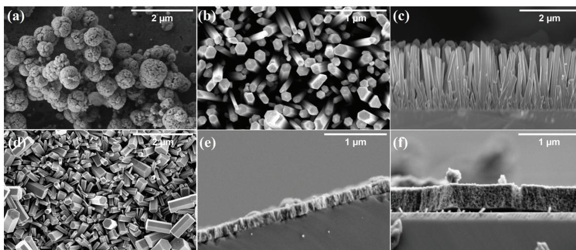
**Figure 1.** (a) Microspheres obtained with DEA/water; (b, c) top and lateral view of nanowires obtained with HMTA/water respectively; (d) nano and microprism obtained with HMTA and water:methanol 50:50; (e) columnar thin film obtained with DEA/water; (f) microporous thin film obtained with HMTA/methanol.
