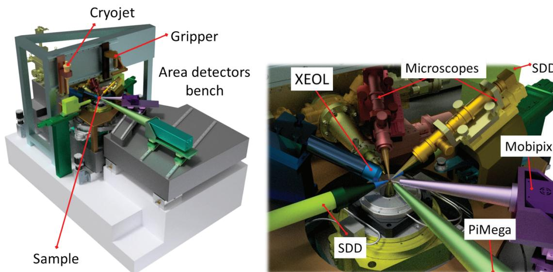
**Figure 6.** Scanning probe TARUMÃ at CARNAUBA nano and microprobe beamline. SIRIUS synchrotron laboratory in Campinas, Brazil. (Figure by courtesy of H. Tolentino, SIRIUS, Campinas, Brazil (H.C.N. Tolentino, R.R. Geraldes, 2019).
