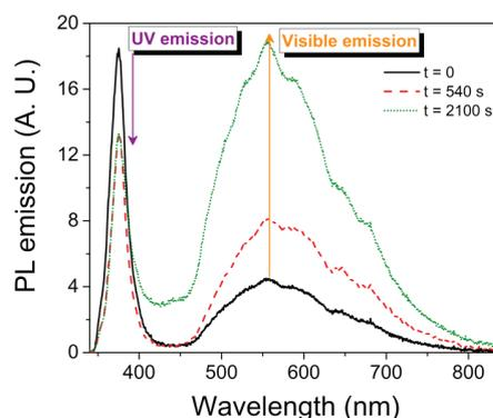
**Figure 2.** Evolution of the photoluminescence spectrum as function of the excitation time for microspheres obtained with DEA/water. The legend indicates the excitation times at which each spectrum was acquired. From [28], copyright IOP.
