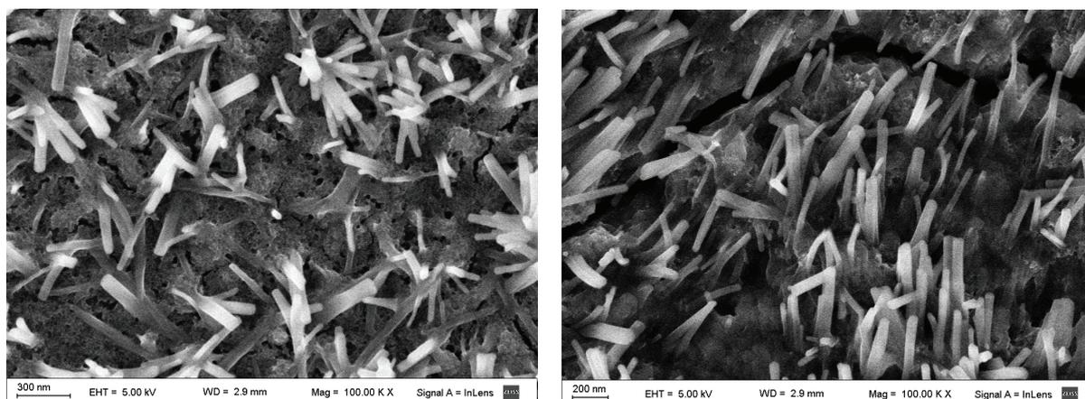
**Figure 5.** SEM micrographs of ZnO nanowires grown in the first stages of deposition by EPD, corresponding to two different zones of the same sample (a and b). It shows the initial appearance of a nanoporous film on which the ZnO nanowires grow. Parameters of applied voltage, electrode-substrate separation and deposition time were 33 V, 7.5 mm and 40 minutes, respectively. SEM micrographs at 100 KX of magnification.
