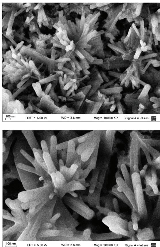
**Figure 4.** SEM micrographs at different magnifications a) 100 KX and b) 200 KX, of ZnO nanowire bunches, grown on p-type crystalline Si doped with B <100> substrates, with resistivity (1-10)  $\Omega \text{ cm}$ . Optimum parameters of applied voltage, electrode-substrate separation and deposition time were 33 V, 7.5 mm and 1 h, respectively.
