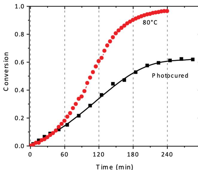
**Figure 15.** Conversion vs. time curves for the epoxy blend with 10 wt% PEB-*b*-PEO, during thermal polymerization at 80 °C (circles) and photocuring at room temperature (squares). [Puig, J.; Ceolín, M.; Williams, R. J. J.; Schroeder, W. F.; Zucchi, I. A. *Soft Matter* **2017**, *13* (40), 7341–7351] Reproduced by permission of The Royal Society of Chemistry.
