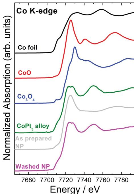
**Figure 2.** XANES spectra at the Co-K edge of as-prepared and washed samples compared to metallic Co foil, CoO, Co<sub>3</sub>O<sub>4</sub> and CoPt<sub>3</sub> alloy reference compounds. Note the energy edge position of samples coincident with metallic Co foil reference and the similarity between the washed sample and the CoPt<sub>3</sub> alloy reference compound.
