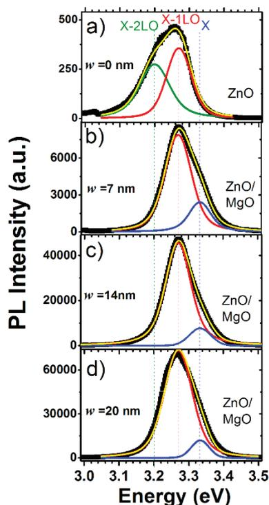
**Figure 7.** Experimental (black symbols) and fitted (yellow lines) PL spectra from ZnO (a) and from ZnO/MgO core/shell NW samples (b, c, d), for different MgO shell widths,  $w$ , in the UV region (NBE band). The components of the fits attributed to the excitonic emission (X) and its phonon replica (X-1LO, X-2LO) are indicated by vertical dashed lines (positions) and by blue, red, and green, respectively. Note the very different vertical scales in (a, b, c, d). From<sup>76</sup>.
