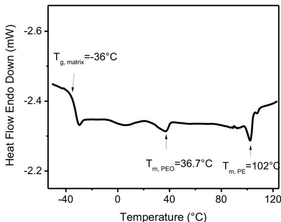
**Figure 5.** DSC thermogram in heating scan at  $10^\circ\text{C}/\text{min}$  of the initial 10 wt % PE-*b*-PEO/DGEBA blend.
