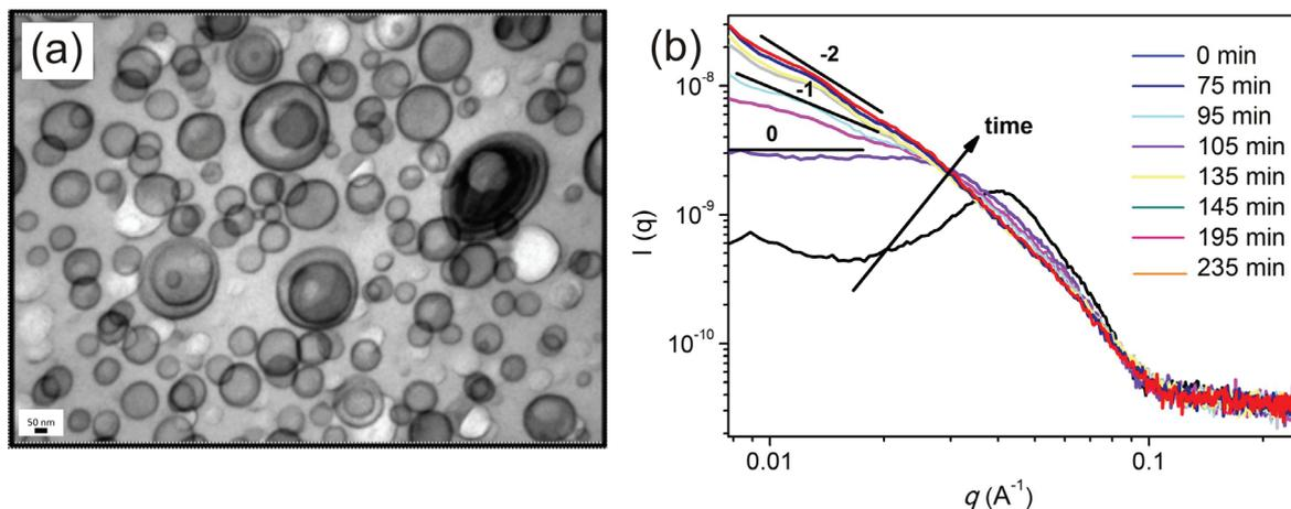
**Figure 14.** (a) TEM image of the epoxy blend with 10 wt % PEB-*b*-PEO photocured at room temperature. The specimen was stained with RuO<sub>4</sub> prior to TEM observation. Scale bar 50 nm. (b) *In situ* SAXS data obtained during photo-polymerization at room temperature of the epoxy blend with 10 wt % PEB-*b*-PEO. [Puig, J.; Ceolín, M.; Williams, R. J. J.; Schroeder, W. F.; Zucchi, I. A. *Soft Matter* **2017**, *13* (40), 7341–7351] Reproduced by permission of The Royal Society of Chemistry.
