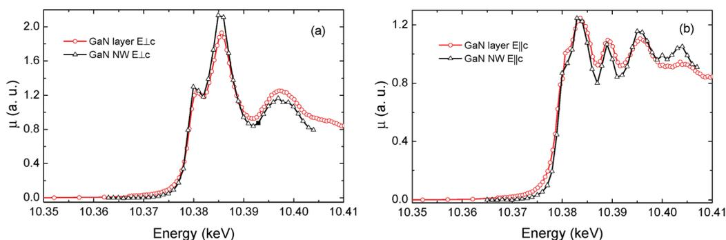
**Figure 9.** Comparison between X-ray absorption near edge structure (XANES) spectra of a high quality reference GaN layer (red circles) and those of the NW (black triangles) for different X-ray beam incident angles: polarization (a) perpendicular and (b) parallel to the wurtzite  $c$ -axis (Figure published with permission of Secco *et al.*, 2019).
