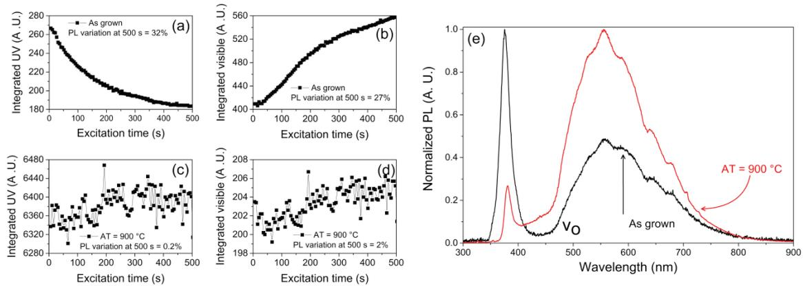
**Figure 3.** PL evolution for microspheres obtained with DEA/water after annealing at 900°C in air. (a, b) integrated emission intensity from the as-grown sample, (c, d) integrated emission intensity from the sample annealed at 900°C for 1 h. (e) PL spectra for the as-grown (black) and annealed (red) samples. From<sup>28</sup>, copyright IOP.
