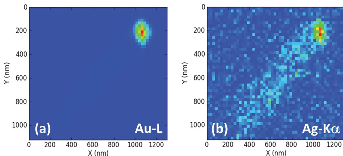
**Figure 8.** XRF colour map distribution of (a) Au and (b) Ag along a representative NW. The colour scale represents the XRF intensity in photon counts and ranges from 0 to 9000 (for Au) and from 0 to 25 (for Ag) (Figure published with permission of Secco *et al.* (2019)).
