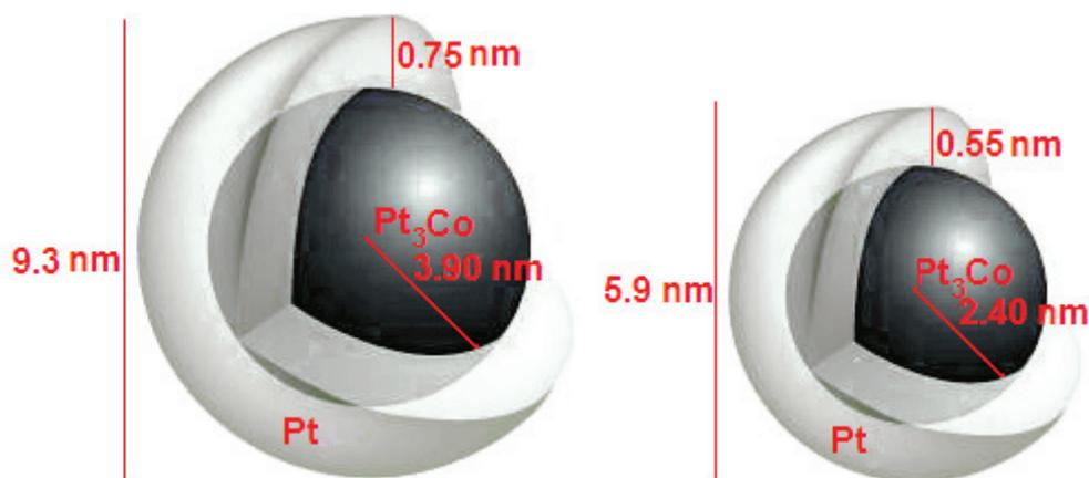
**Figure 4.** Representation of the proposed core@shell structure for as-synthesized and washed NPs (left and right respectively) derived from EXAFS fittings and XANES spectra, compatible with calculated averaged coordination number for determined structures.
